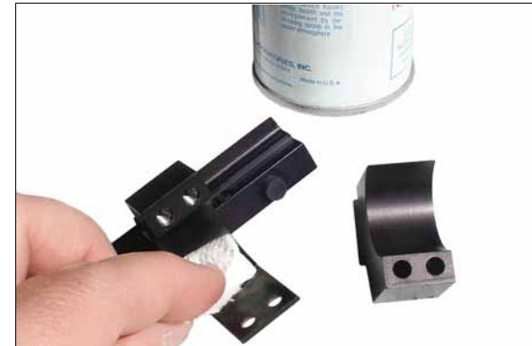
Step 3 - De-grease the interior curved surfaces of both the primary and secondary mounting blocks. Also de-grease the area on the barrel where the I-Mount is to be installed.
