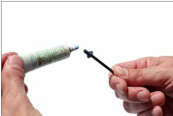
B. Place blue (not red ) Lock-tite on the screw.
