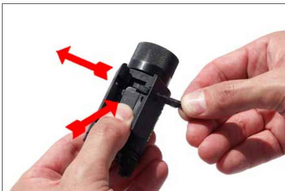
Step 3 - Depress the spring and, from right to left, insert the replacement locking bar. Release the spring to lock the bar in place.
