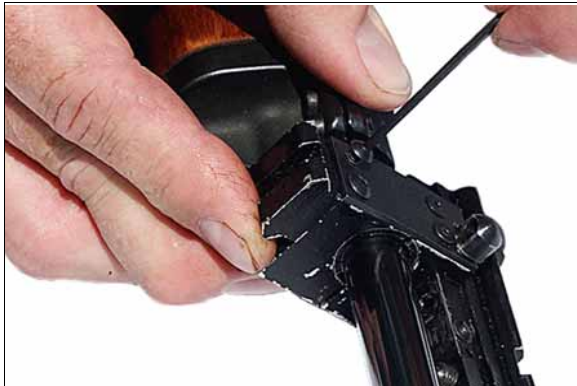
A. Remove only one top plate cap screw.
