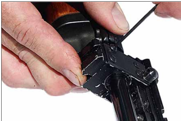
C. Replace & firmly tighten top plate cap screw. Then repeat for the other cap screw.
