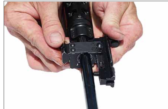
Step 13 - Re-check the alignment of the mount, and ensure the mount can neither move nor rotate.
