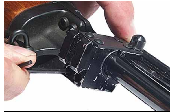
Step 12 - Repeat the Step 11 process using the shoulder screws – remove a screw, coat it with blue Lock-tite, replace and tighten the screw firmly , and then repeat for the other shoulder screw.
